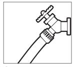
**Step 3** Connect garden hose to the cold water source and turn water on completely.
